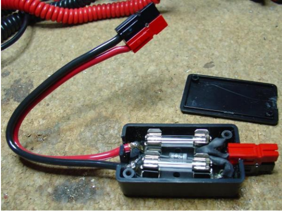
Photo C: Internal view of fuse assembly
